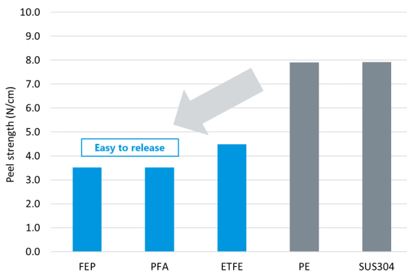
Fig.1 Peel strength of polymer film from metal substrate (Testing methods : JIS Z 0237)
